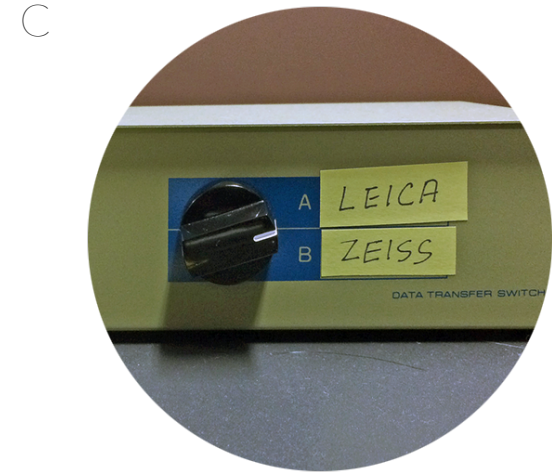
Toggle Laser selector to position A - 'Leica'.
